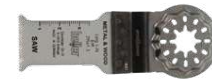
BIM Metal & Wood Saw, 50 x 28 mm Wave universal teeth. Iron sheet, aluminium, Copper, Wood, Gypsum, Plastic. High Speed. Art.-Nr. 29541 3 & 29542 0
